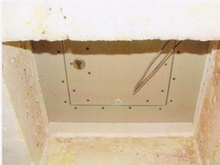
Photo 2: flaming from the underside – test sample from the fire side before the fire test
